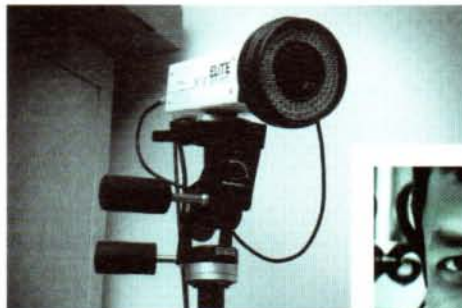
Delphine's motion capture system uses four infrared cameras (above) positioned in the corners of a room
